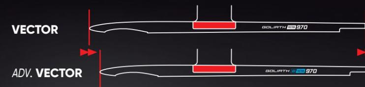
> **ADV = Advanced** : the mast mounting footprint is advanced on the fuselage.
